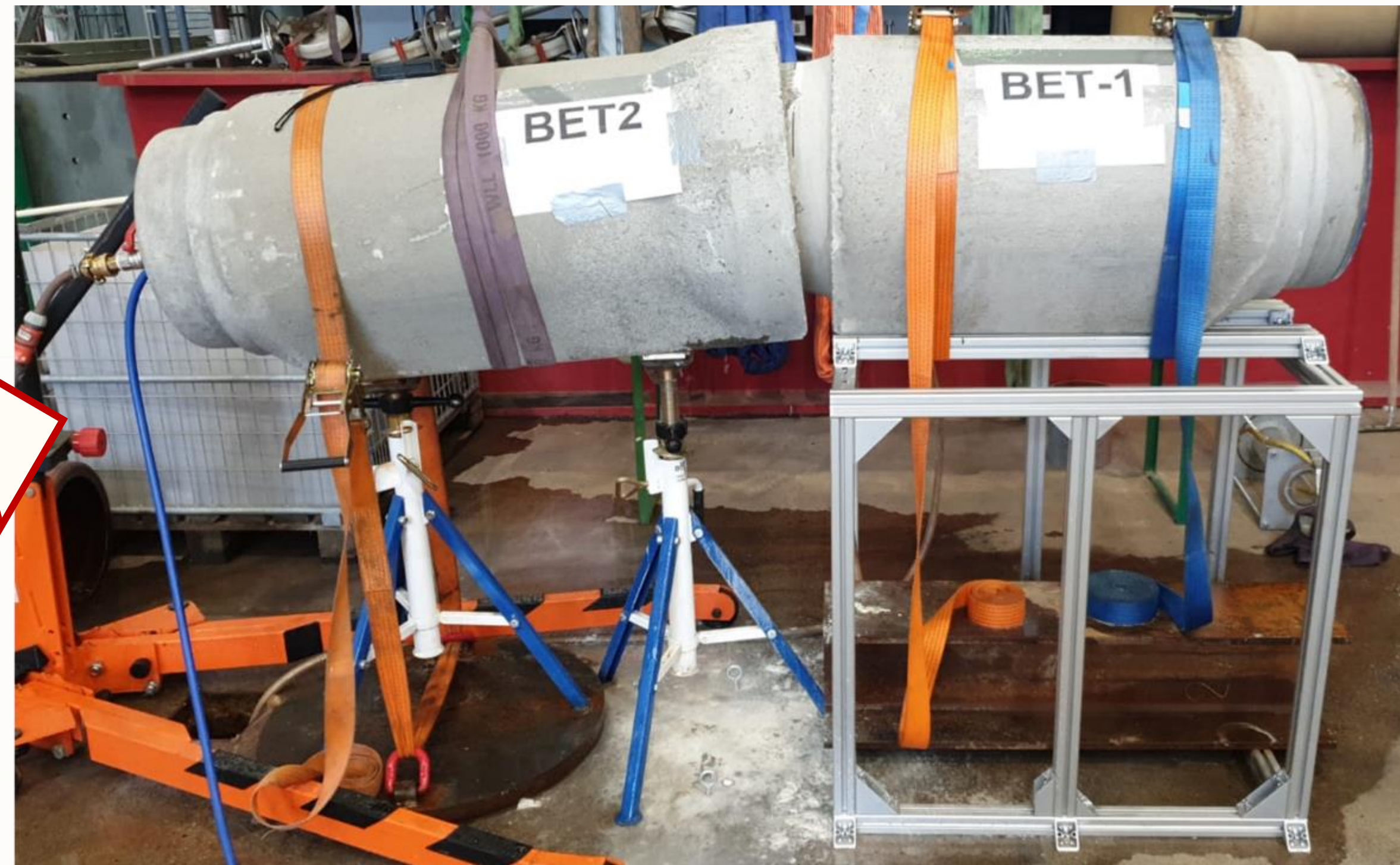
Lab exfiltration test setup at IKT
