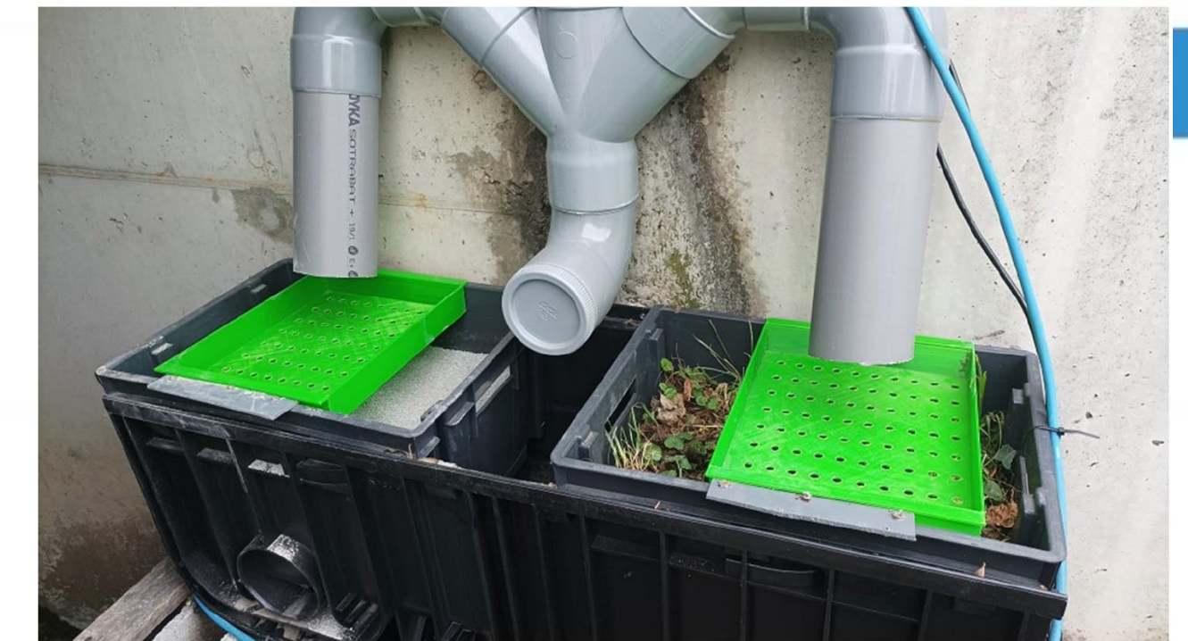
Sampling and chemical analysis: Dissolved organic carbon (DOC) and Heavy metals concentrations at the inlet and outlet of substrates
